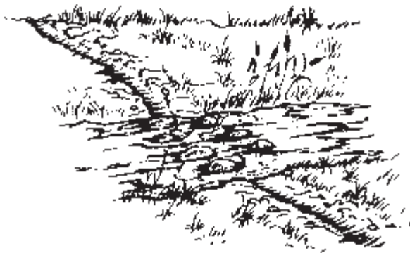
Flat stones work as effective materials for creating paved stream crossings.
